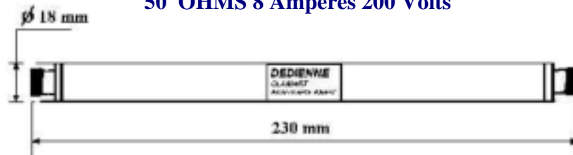
Specially Adapted filter 50 OHMS 8 Amperes 200 Volts
